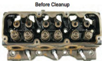
Cylinder head pre-cleanup. Note the sludge deposits on and around the valve springs and push rod openings.
