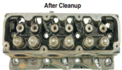
Cylinder head after cleanup with AMSOIL Engine and Transmission Flush. The valve springs and push rod openings are noticeably cleaner, with fewer sludge deposits. The manufacturer's stamping is more easily seen.
