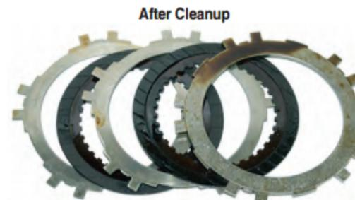
Automatic transmission clutch plates after cleanup with AMSOIL Engine and Transmission Flush reveal lighter glazing and varnish.
