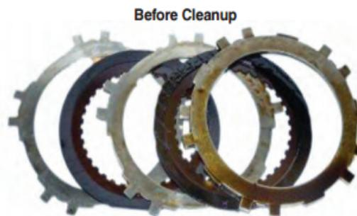
Automatic transmission clutch plates pre-cleanup. Varnish and glazing is heavy on some of the plates.
